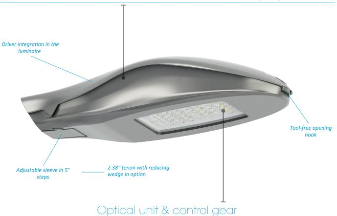
16 to 48 LED module in Zhaga standard - From 1000 to 13800 lm (see attached EVO2 data sheet for details on power, light intensity and photometry available). Integrated smart driver (control, automatic adjustment, CLO, graduation via voltage variation or DALI). ULR 0% (LED) (ULR: Upward Light Ratio).
